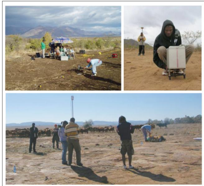
**Figure 1.** Students in the geophysics field course collecting seismic refraction data (top left), gravity data (top right), and magnetic data (bottom).
