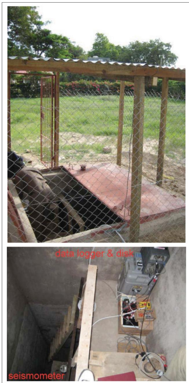
**Figure 3.** A permanent AfricaArray seismic observatory in Tanzania. (top) Security fence and metal lid covering a vault whose depth is 4 m. (bottom) Interior of the vault.
