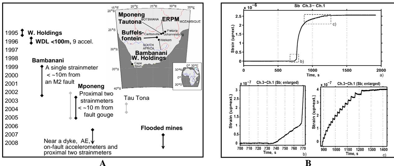
**Figure 1** A. Semi-controlled Earthquake-generation Experiments in deep South African gold mines up to 2008 (after Ogasawara et al., 2009). B. Slow strain changes with a clear forerunner (735 s to 765 s) observed at the Pretorius fault zone, Mponeng mine (after Ogasawara et al., 2009; data after Yasutake et al., 2006).
