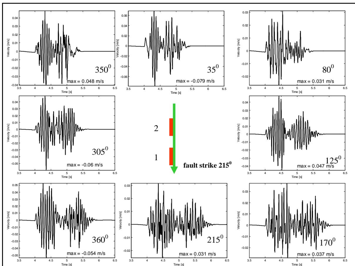
**Figure 5** Velocity of ground motion predicted at a distance of 5 km from the epicentre on a hard rock surface. The station azimuth is displayed next to each synthetic seismogram. The fault strike was  $215^\circ$ . The positions of two asperities are marked with bold lines.
