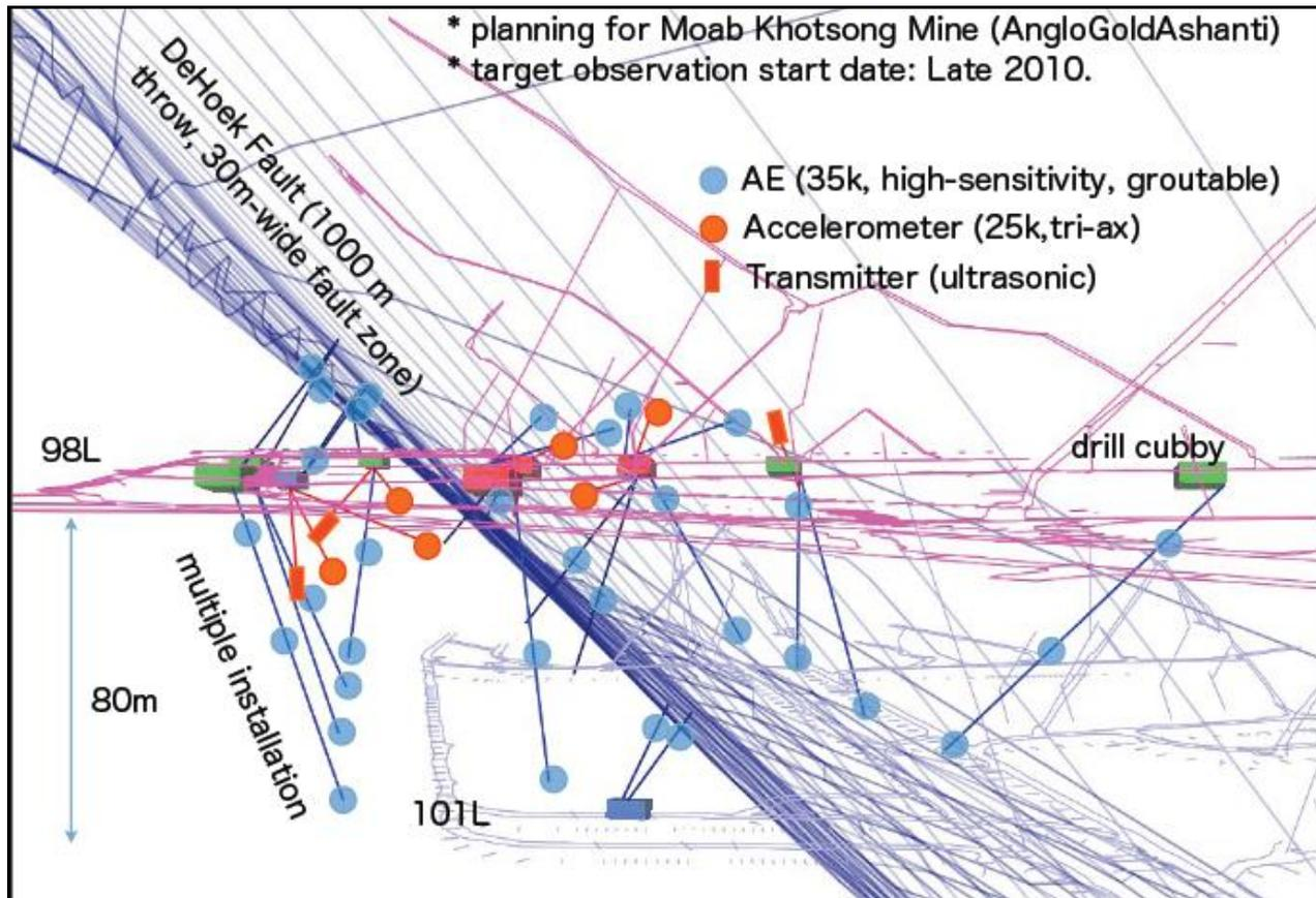
**Figure 6 Monitoring instrumentation planned for Moab Khotsong Mine, Klerksdorp gold field**
