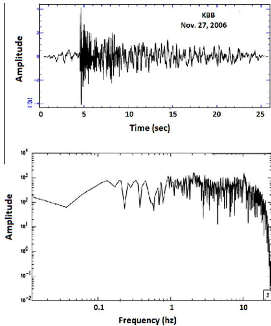
**Fig. 2.** Velocity spectra of typical hybrid (LP + short) events (27 November 2006). The lower and upper corner frequency of the instrument (Trillium 40) are 0.025 Hz and 50 Hz, respectively. The Nyquist frequency is 25 Hz.
