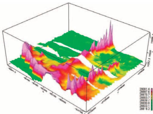
**Figure 6.** Magnetic data collected over intersecting dykes on a mine property. The change in amplitude of the magnetic signal clearly indicates a change in overburden thickness. Figure courtesy of Ralf Hansen, 2007.
