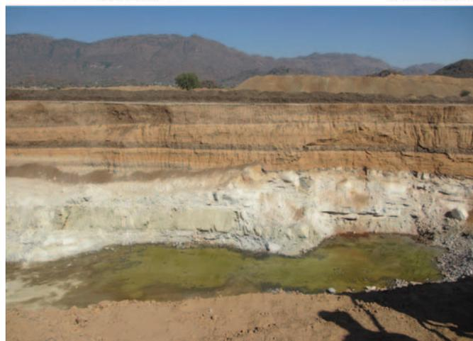
**Figure 5.** Open-pit mine with layered sediments in brown and fresh norite lithologies underneath. The resistivity line was collected the previous year perpendicular to the pit face at about position 150 m.
